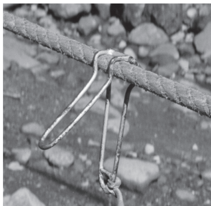
A New Zealand rope tow “nutcracker” as commonly used around our skifields, and a US de luxe version which is on display in Colorado.
